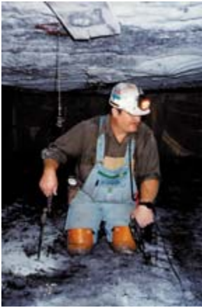
Jim Kilgore preparing to use a right angle prism for setting a drive spad.
