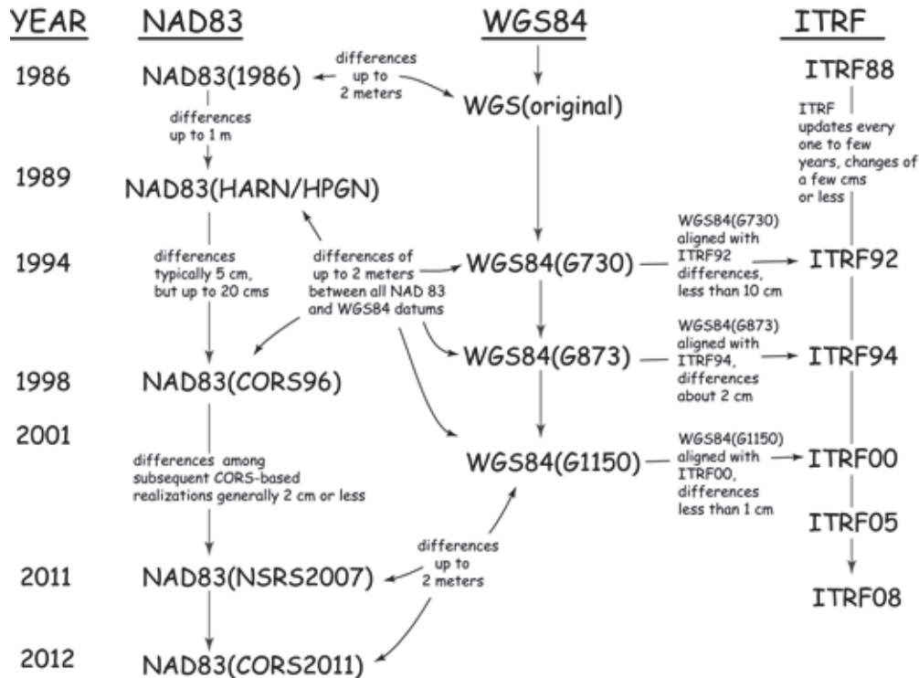
Figure 3-23: This graphic summarizes the evolution of the three main families of datums used in North America. As the datums have been adjusted, horizontal positional differences between bench mark points have varied, within the ranges shown. “Aligned” datums (e.g., WGS84(G1150) and ITRF00) may be considered equivalent for most purposes when applying datum transformations.
