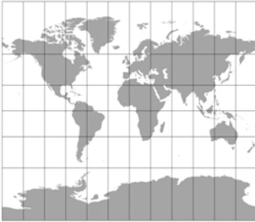
Figure 3-46: A Miller cylindrical projection, commonly used for maps of the world. This is an example of an uninterrupted map surface.
