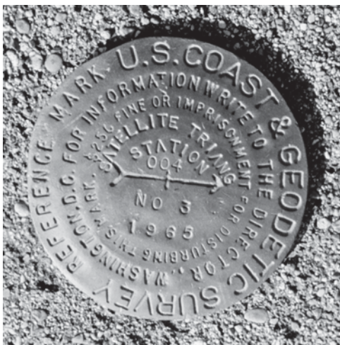
Figure 3-15: A brass disk used to monument a survey bench mark.
