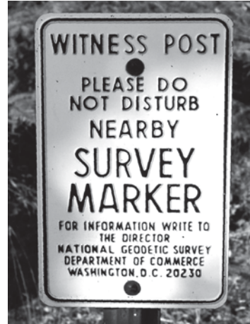
Figure 3-16: Signs are often placed near control points to warn of their presence and aid in their location.
