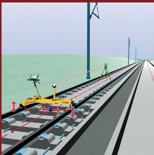
The Amberg slab track application provides guidance for right rail, left rail and planimetric position of track.
