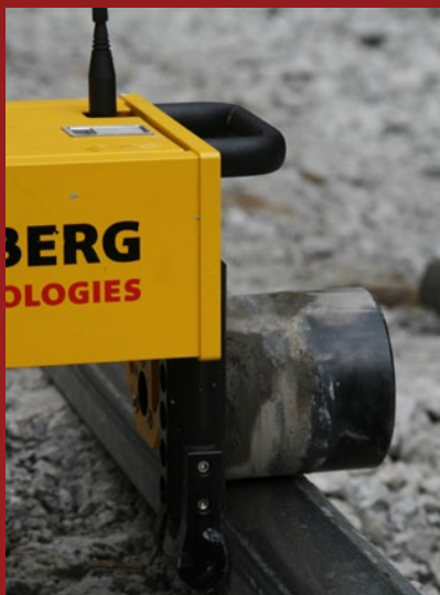
The gauge sensor of the Amberg GRP provides measurements accurate to +/- 0.3mm
