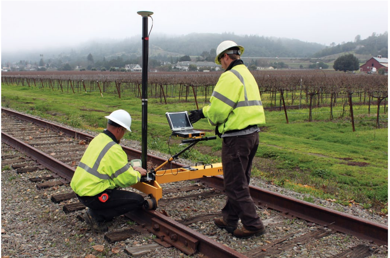
CPI Surveyors James Brown (L) and Erik Vonderscheer (R) prepare the Amberg GRP for measurement.
